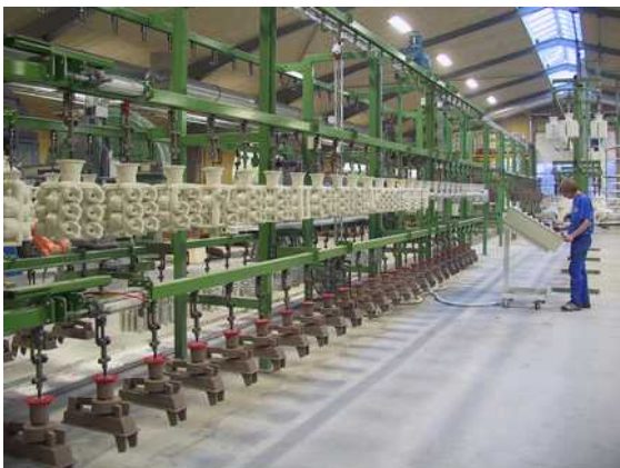
Fully automatic moulding-line
