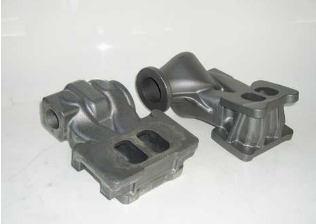
Turbo Exhaust parts - EN-GJS-XSiMo 5.1 – Shellmould
